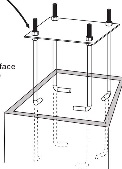
**YOU ARE NOW FINISHED WITH THE INITIAL ASSEMBLY STEPS. DO NOT PROCEED WITH THE ASSEMBLY UNTIL THE CONCRETE HAS FULLY CURED. CURING WILL TAKE A MINIMUM OF 72 HOURS. IN HUMID CLIMATES OR WET WEATHER, ALLOW ADDITIONAL TIME FOR THE CONCRETE TO CURE.**
