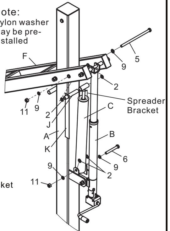
**C.** Remove and discard the spreader Bracket from the Spring Cartridge.
